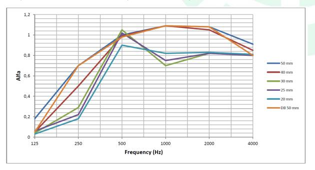
Testing of Whisper<sup>®</sup> was done at Istituto Giordano, Bellaria in Italy. Testing was carried out under EN ISO 354:2003 Measurement of Sound Absorption in a reverberation room.
